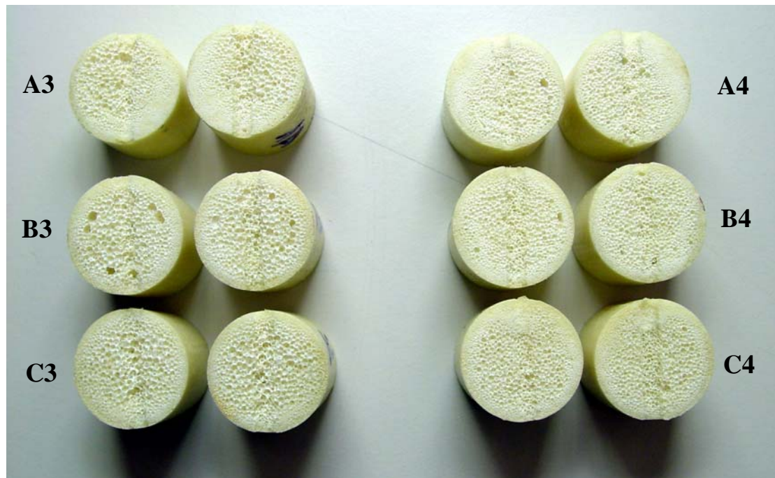
Figure 10: Cross sections of the bone samples A3, B3 and C3 (left, from top to bottom) and A4, B4 and C4 (right, from top to bottom) at the screw insertion site. Specimens A4, B4 and C4 had a higher pull-out strength because of the lower porosity of the foam material compared to the other specimens.
